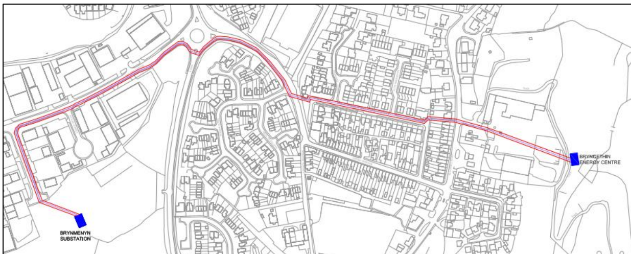
Figure 8: Line of Private Wire Connection
